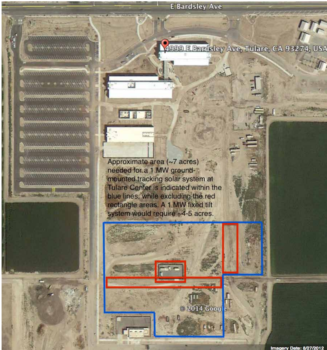
Exhibit 1: Aerial Photo of the proposed Placement for Possible Ground-mounted Solar Panel Project at Tulare College Center.
